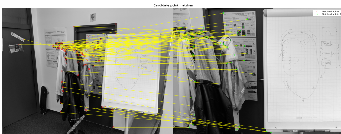
Figure 6: Matches calculated by SIFT descriptors.
